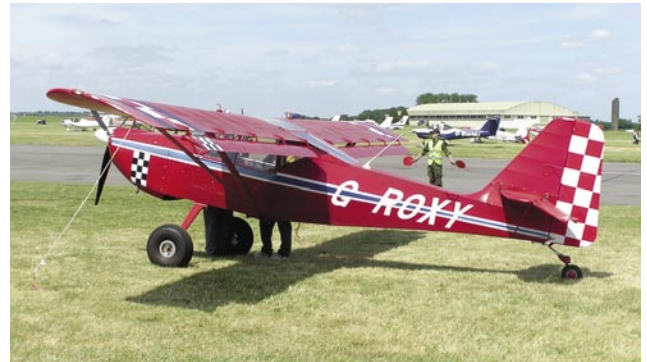
Figure 5-9. Flaperons on a Skystar Kitfox MK 7.
