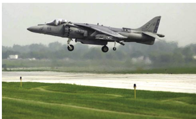
Figure 4-4. Some aircraft have the ability to change the direction of thrust.
