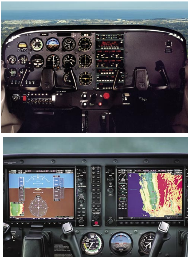
Figure 2-18. Analog display (top) and digital display (bottom) from a Cessna 172.
