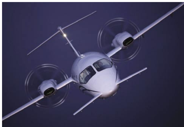
Figure 5-14. The Piaggio P180 includes a variable-sweep canard design, which provides longitudinal stability about the lateral axis.
