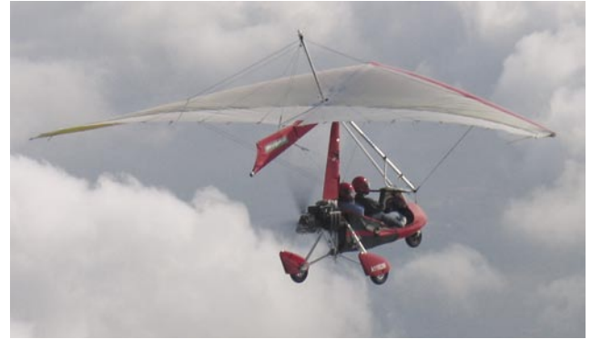
Figure 2-9. Weight-shift control aircraft use the shifting of weight for control.
