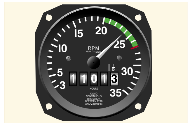
Figure 6-8. Engine rpm is indicated on the tachometer.
