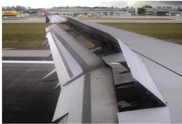
Figure 5-19. Spoilers reduce lift and increase drag during descent and landing.
